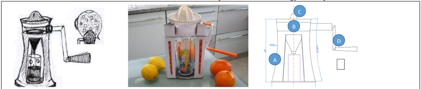
Figure 5. From concept, in the left, to a looks like prototype in the centre and to detail design, in the right (Adapted from [22]).
